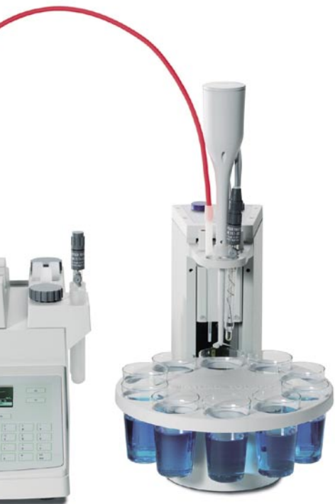
A DL50 Titrator with a Rondolino sample changer determines alkalinity in mineral water, acid number in soft drinks and concentration of alkaline cleaning fluid.
