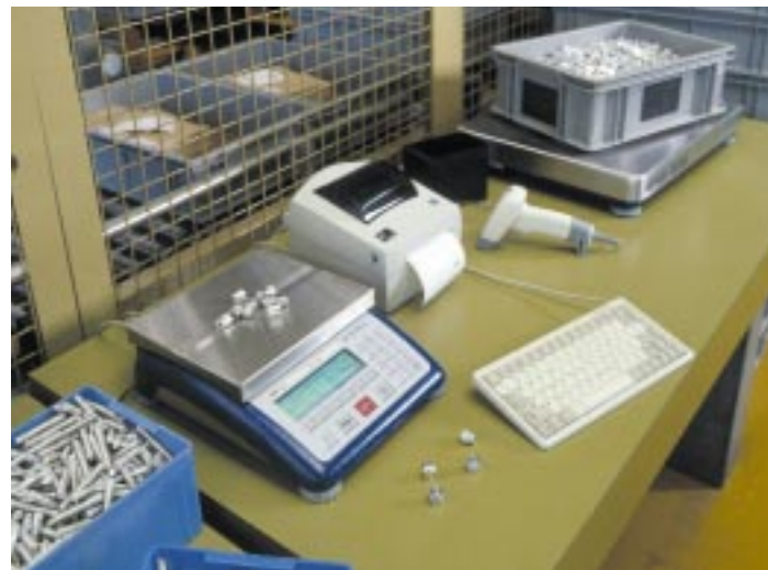
Two-scale system: Viper SC as reference scale and analog weighing platform as quantity scale
